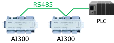
Connection via RS485
